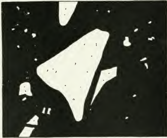
Fig. 20—Character of ore at Creighton mine, Sudbury area, Ontario, eighth level, 10 feet from hanging wall. White represents rock; black represents sulphides. Width of face 5 feet.
